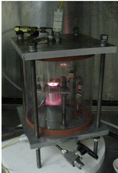
**Figure 8 - High Temperature Controlled Atmosphere Furnace**
