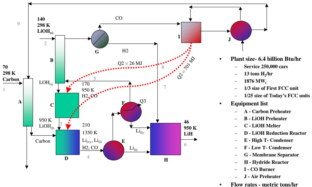
Figure 6 - Simplified ASPEN Plus Process Flow Sheet
