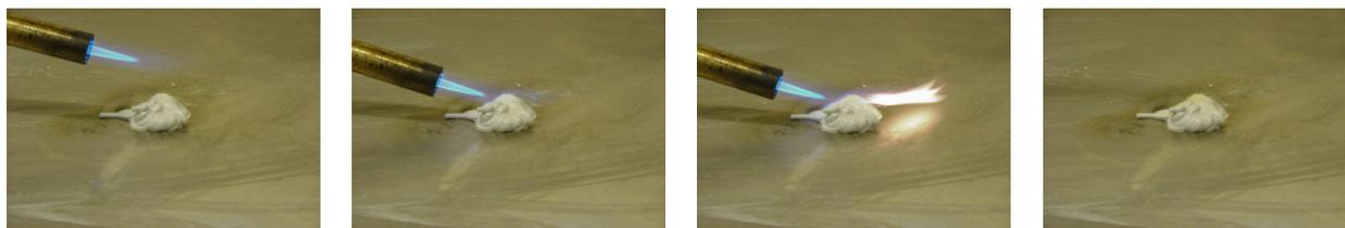
**Figure 4 - Flame Test with LiH Slurry**
