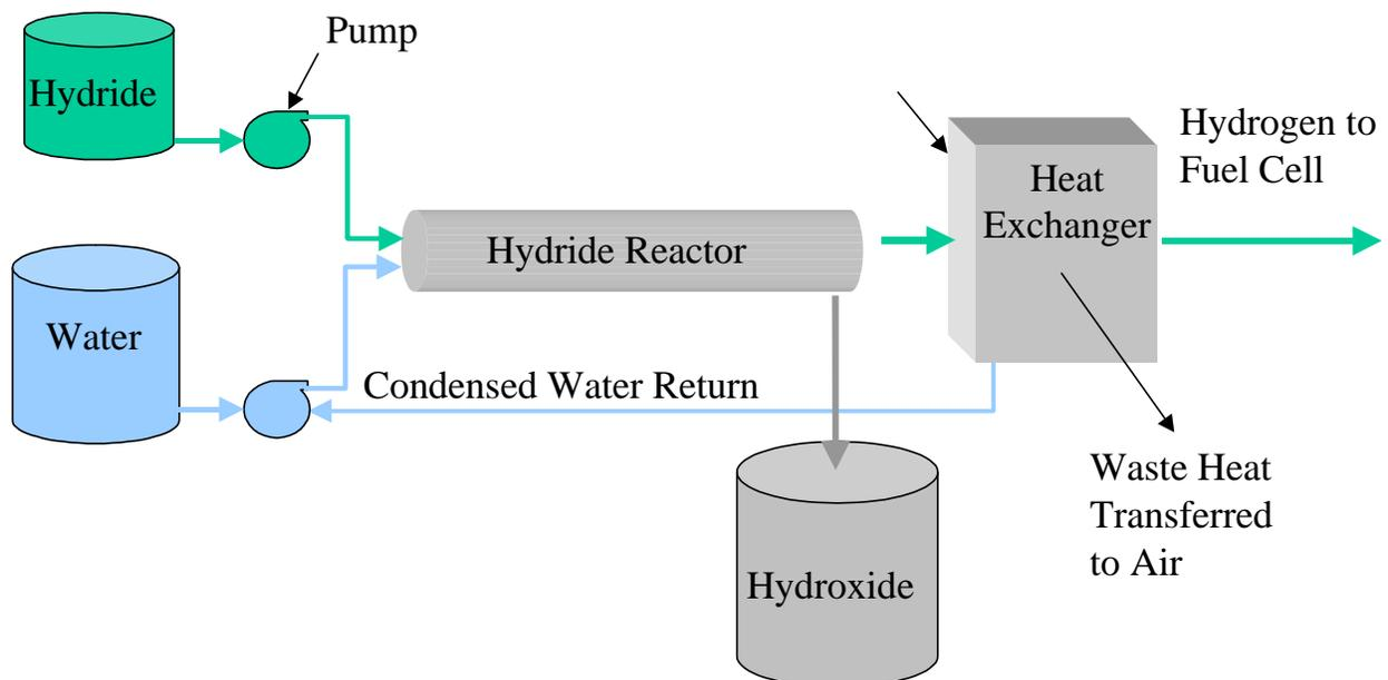
**Figure 12 - Diagram of the Hydrogen Generation System**
