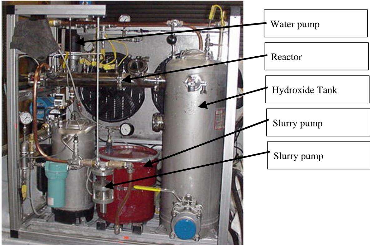
**Figure 13 - Picture of the Prototype Hydrogen Generator**
